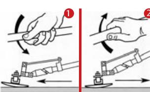
1. Its mechanism allows, through a simple turn of the handle to the right, to make the blade incline forward, pushing and spreading the concrete.
